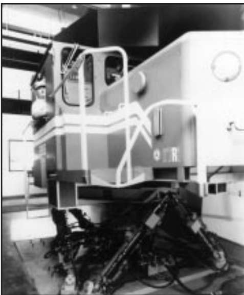
Research and Locomotive Evaluator/Simulator (RALES) Courtesy of IIT Research Institute, Chicago IL
